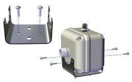
The PE202 may be supported by its piping connections **IF** the piping is rigid. The meter and pipe must be perfectly aligned with no flexion at the fittings to prevent leakage or damage to the meter.
